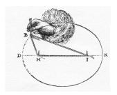
(b) a compass forces one of its points to move at a constant distance from the other one; in the so-called "gardener's device", the sum of the distances of the pencil from two pins remains the same at any moment.
